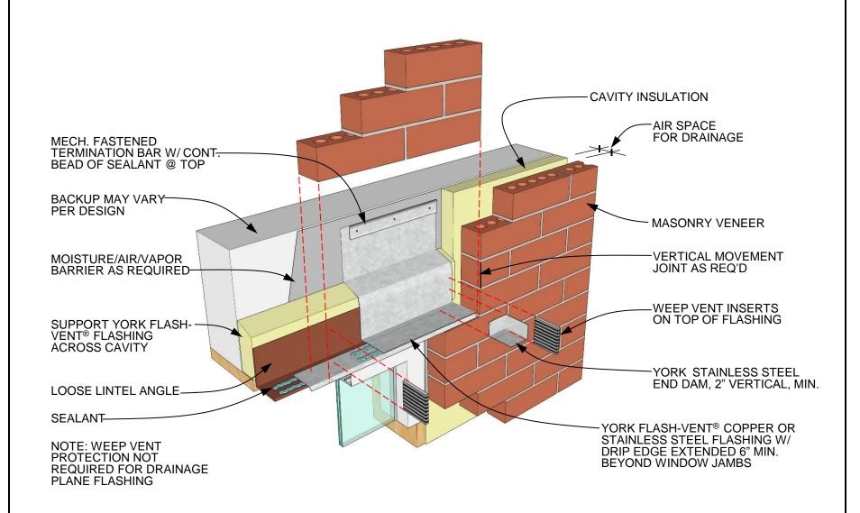
WINDOW HEAD DETAIL YORK FLASH-VENT® FLASHING W/ TERM. BAR DRAWING NO. 04-04 REV. 12/23/14
